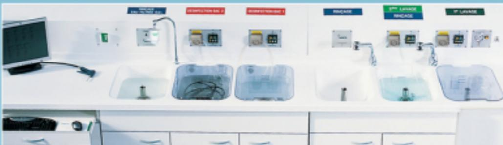
The 6-tray module allows the treatment of 4 endoscopes simultaneously. Work offset from right to left.
